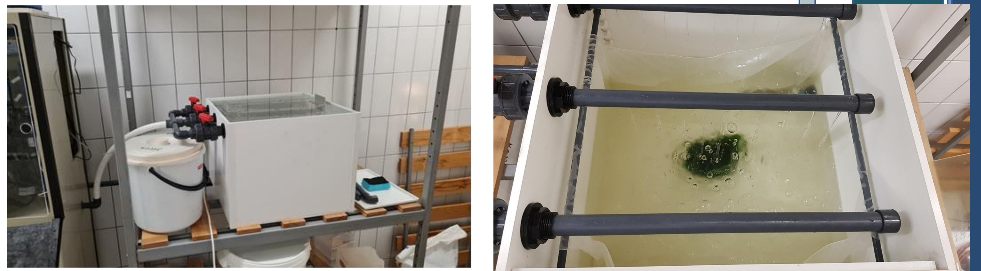
Fig. 1-2. The example of refugium for algae growth experiments.
